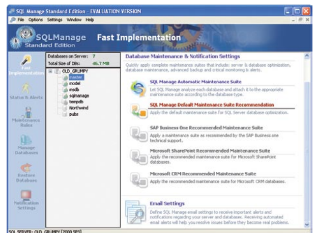
Figure 1: Using the Fast Implementation option to set default maintenance for a database
